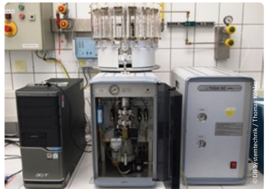
Fig. 3: Measurement setup for gas-in-oil analysis
