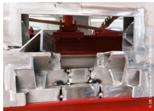
Solebar repaired on the basis of the 3D model
