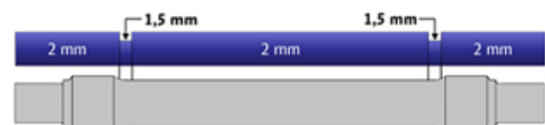
Fig. 3: Areas with a lower detection threshold to extend the UT test interval
