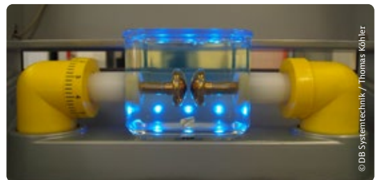
Fig. 2: Determination of the breakdown voltage
