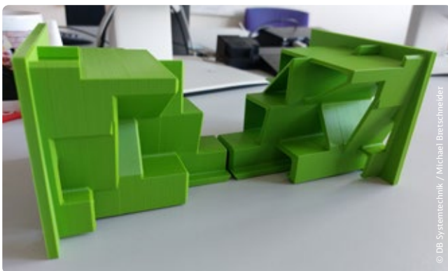
3D-printed model of the solebar repair on a scale of 1:5
