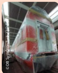
Use of a colouring primer, rendering a clearcoat unnecessary
