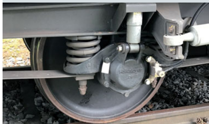
Wheelset in the measuring bogie of the noise monitoring car with accelerometers on the axlebox
