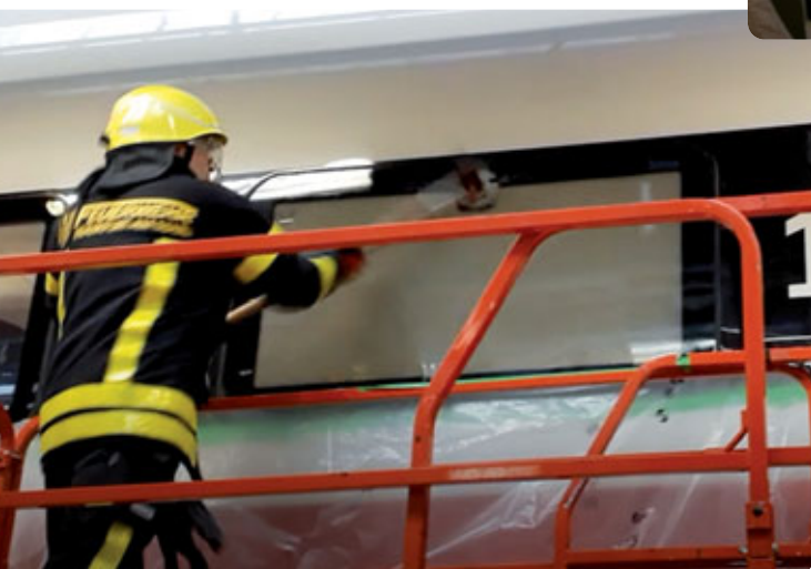
Figures: Window pushed out following functional testing
