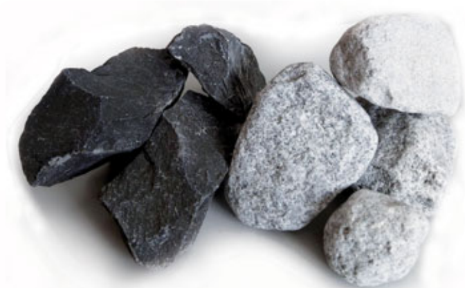
Figure 1: Track ballast before (left) and after (right) an LA test
