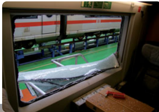
Figures: Window pushed out following functional testing
