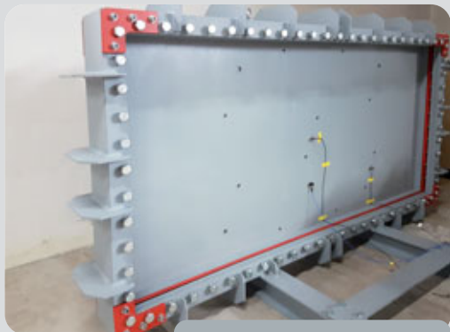
Front of the test system with three vibration pick-ups
